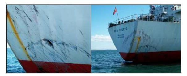
Figure 5.5. Damages of M/V New Breeze (Artena marine Survey)
