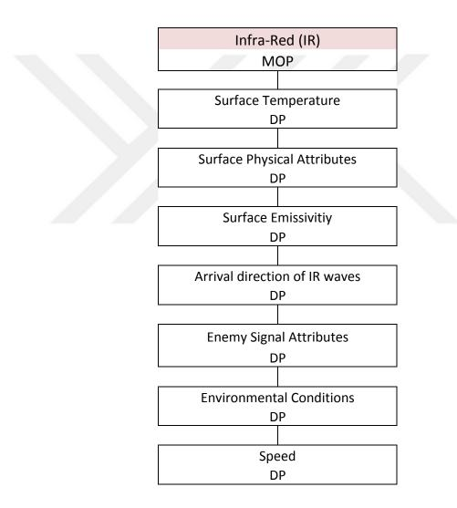
A ships IR signature consists of two main components, which are the heat created by the ship itself and the effect of heat sources of ship's surroundings. Heat rising is caused by thermal radiation in the electromagnetic spectrum particularly in wavelengths. All objects emit IR radiation although hotter objects emit IR with greater intensity. The amount of
