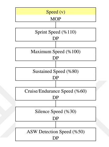
As mentioned before, speed is one of the three main parameters in survivability focused warship design. Design shouldn't be fixed around a certain "speed", but should consider multiple speed levels achievable by the selected machinery for different necessities of different missions assigned by the associated navy.
