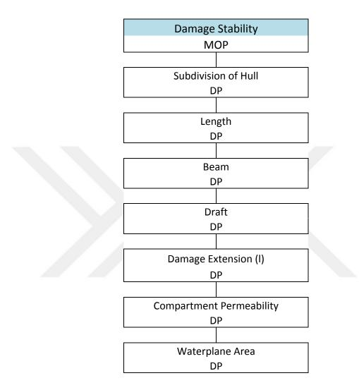
Damage stability criteria must be compatible with intact stability criteria. It is very beneficial to do damage length calculations during predesign to eliminate damage stability complications. Length and number of compartments are decided upon damaged length calculations provided by class society rules.
