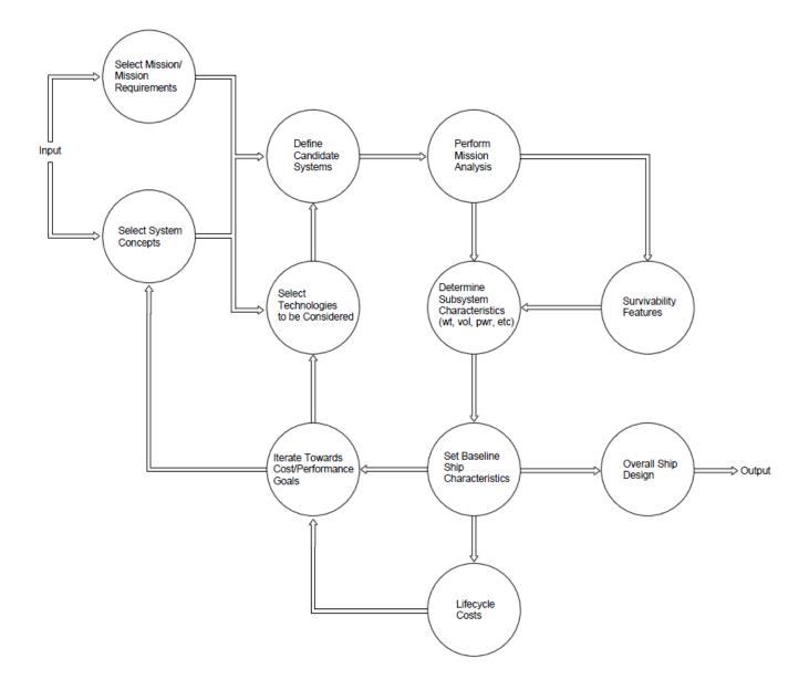
Figure 10.1 - Green's Ship as a Weapons System Diagram
