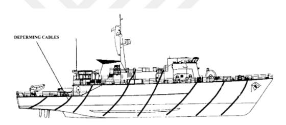
Figure 6.11 - Degaussing System [29]
