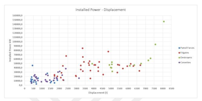
Figure A.4 - Installed Power/Displacement
