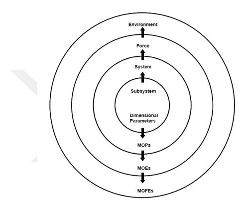
Figure 5.2 - System Boundary Levels [35]
