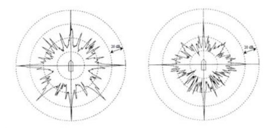
Figure 6.8 - RCS Profiles with and without shaping [11]
