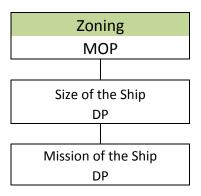
Zoning is important for damage and fire control, in case of losing portions of the ship during war, it must sustain the damage and survive, therefore zoning is utmost important for warships as each zone is able to control the whole warship and its systems on its own.
