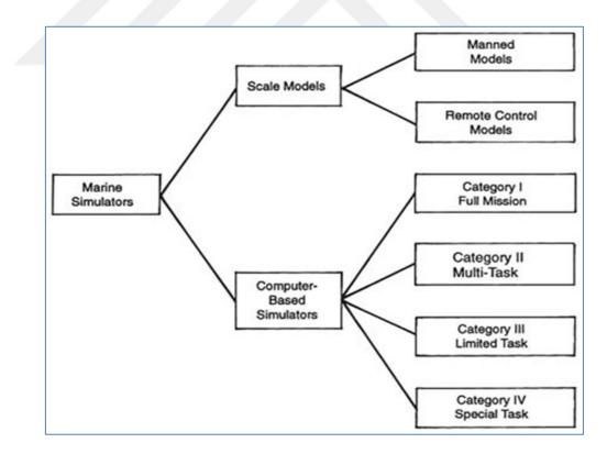
Figure 2: Types of Marine Simulators (Sources: <u>https://www.nap.edu/read/5065/chapter/4#41</u>)
