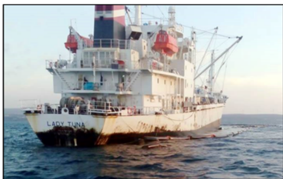
Figure 7. Containment of Spilled Oil by Barriers (www.seanews.com.tr, 2017).
