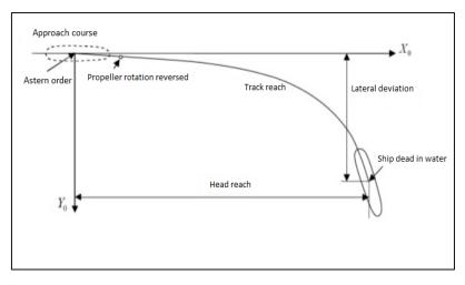
Figure 3.3. Path of ship during stopping ability test (Taha, 2016).
