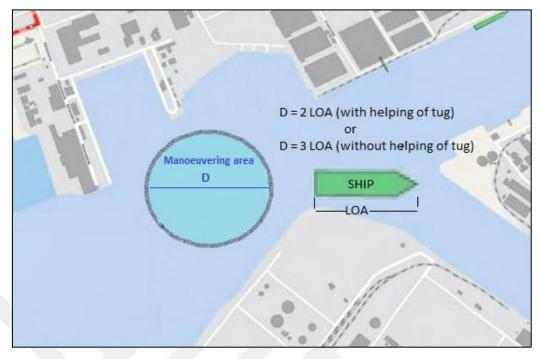
Figure 3.5. Minimum manoeuvring area for ships in port
