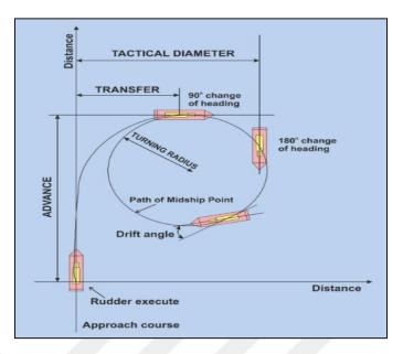
Figure 3.2. Turning circle manoeuvre test (Ghosh, 2019).
