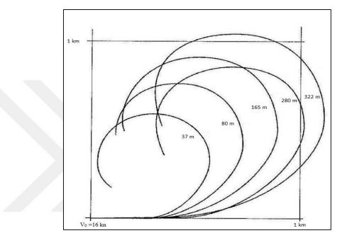
Figure 3.4. Effects of ship's dimension on turning performance (URL-3).
