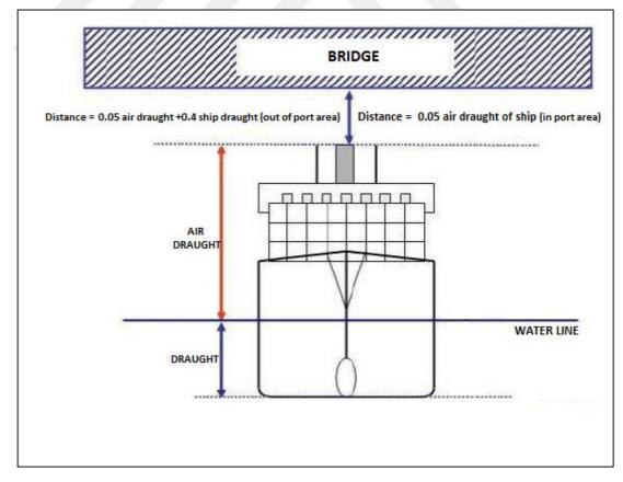
Figure 3.7. Distance between ship and height restriction (PIANC, 2014)
