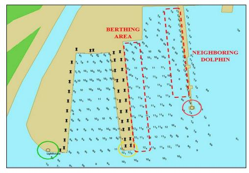
Figure 5.3. 2D model showing the depths of the port
