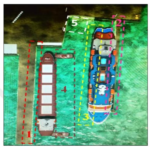
Figure 7.1. Regional distrubition of hazard types that can occur during the model ship is coming alongside to the pier
