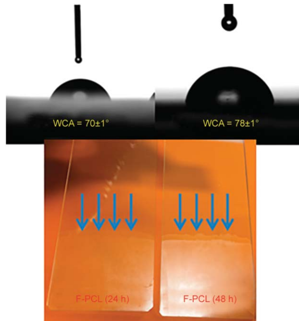
Figure 6. The static contact angle values of water drops on the F-PCL samples, their contact angle pictures, and F-PCL coated glass plate substrates.
