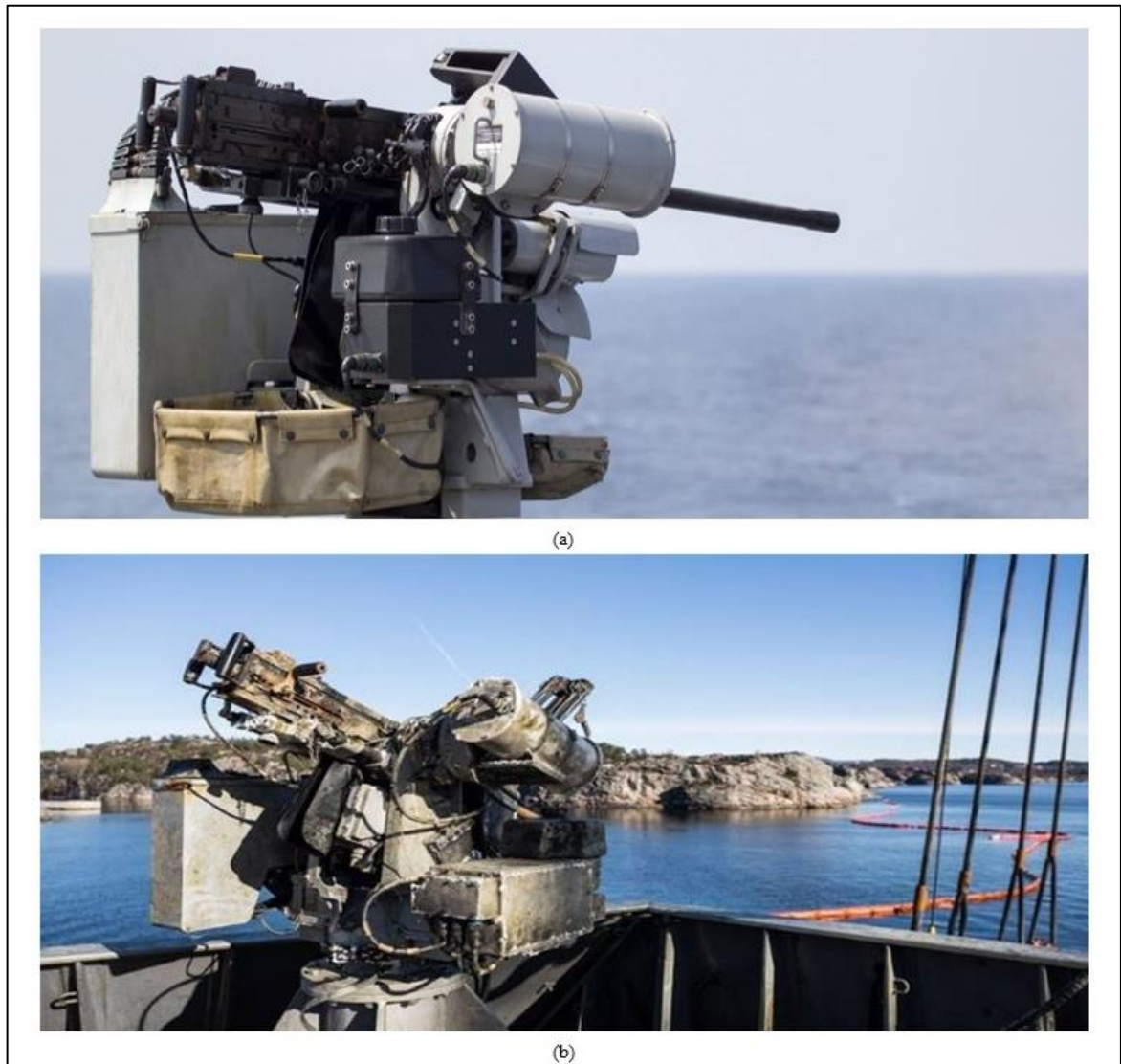
Figure 3.2. Kongsberg Sea protector (a) in normal conditions (b) after spending over 4 months underwater [22].
