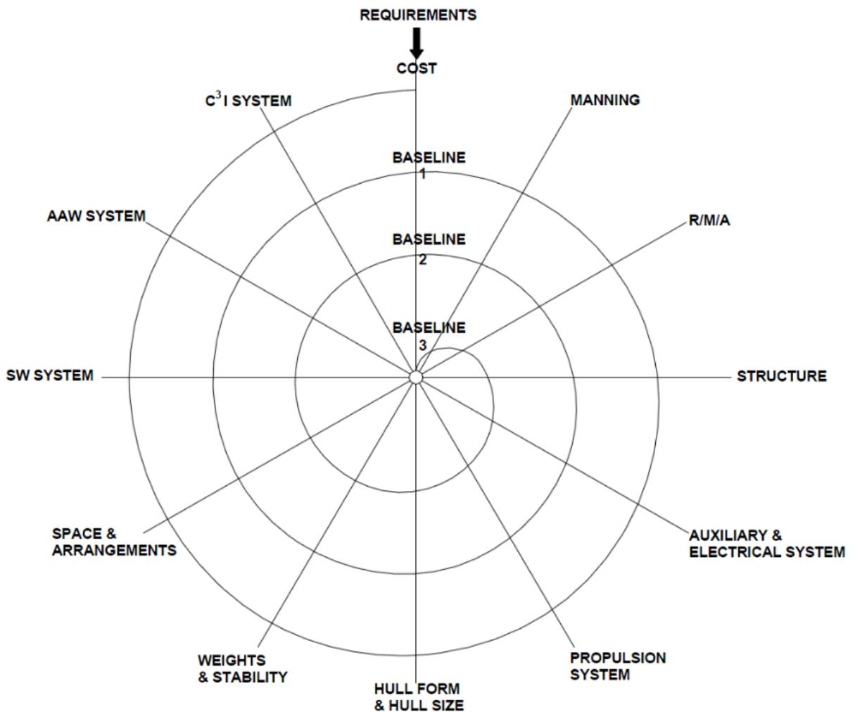
**Figure 6.3 - Combat System Point of View Warship Design Spiral**
