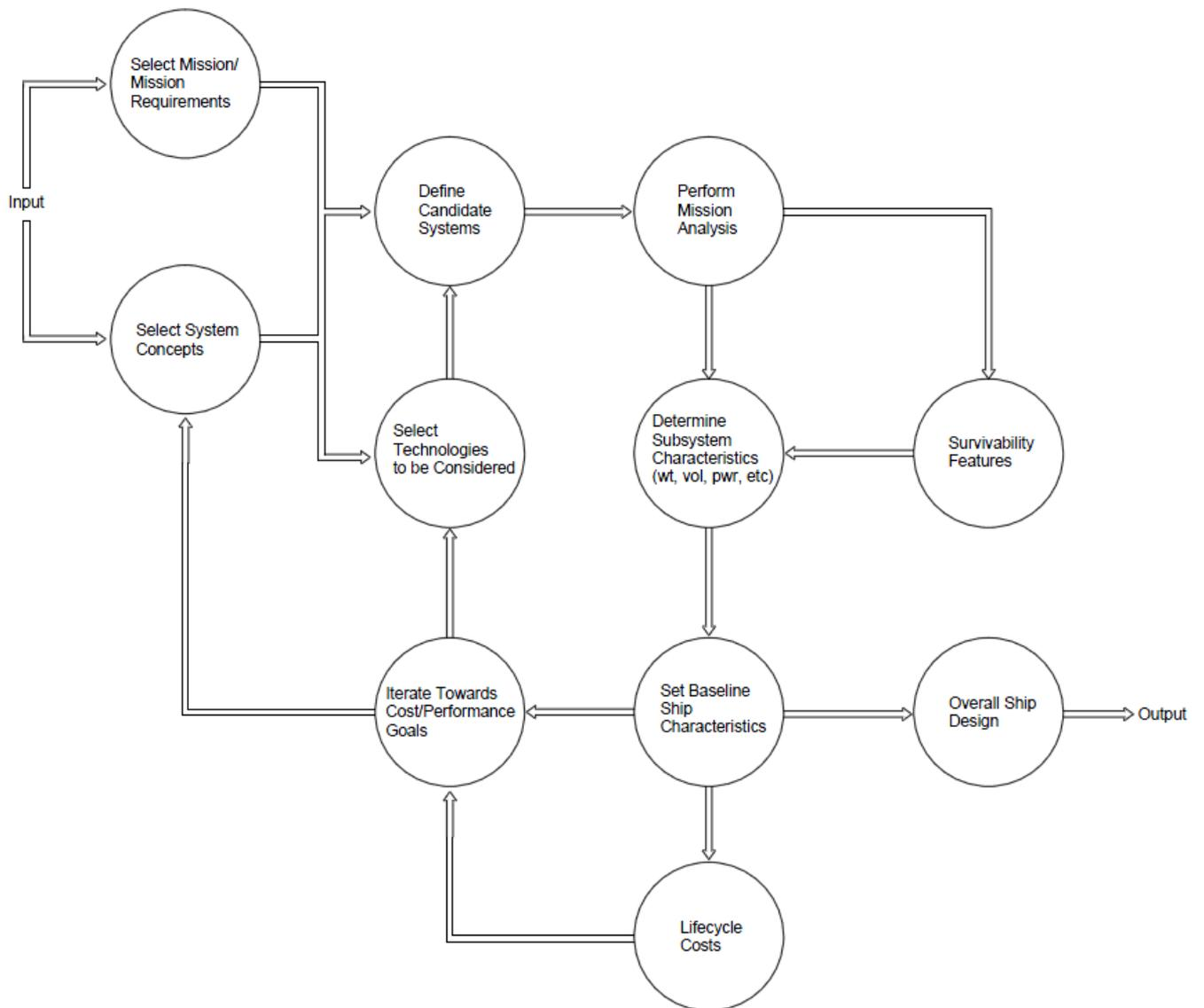
**Figure 10.1 - Green's Ship as a Weapons System Diagram**
