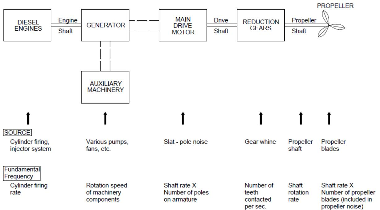
**Figure 6.9 - Schematic Visual of Machinery-borne Noise [24]**
