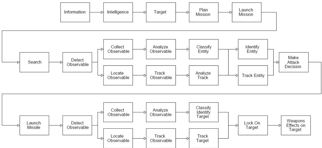
**Figure 6.5 - Anti-Ship Missile Kill Chain [30]**
