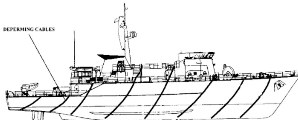
**Figure 6.11 - Degaussing System [29]**
