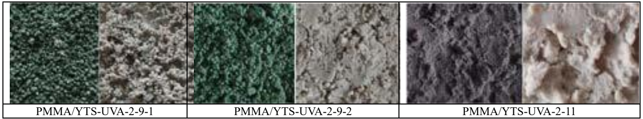
Fig. 1: Colorless (hot) and Colored (cold) photos of the microcapsules
