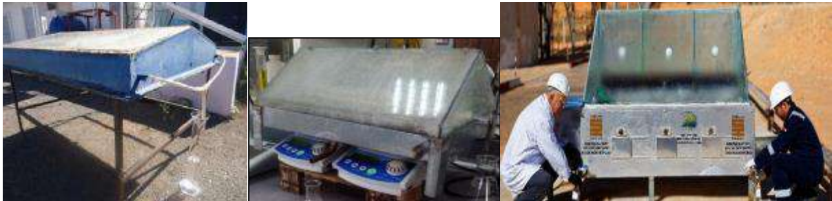
Fig. 1: Greenhouse solar still Fig. 2: Greenhouse hybrid solar still Fig. 3: Greenhouse hybrid multi-sources solar still
