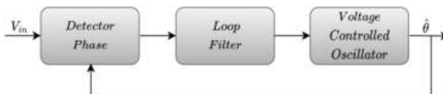
Fig. 1: Block structure of the PLL (Giotopoulos and Korres, 2023)
