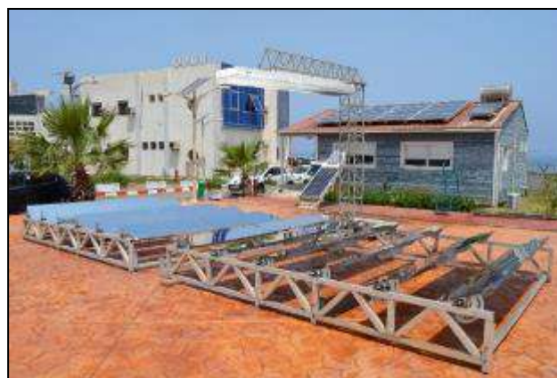
Fig. 3: Fresnel solar concentrator built at UDES
