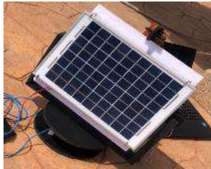
Fig. 2: Two-axis solar tracker system.
