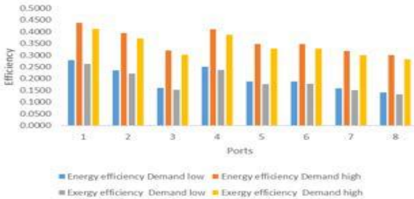
Fig.4 Energy and exergy efficiencies of on-demand ports
