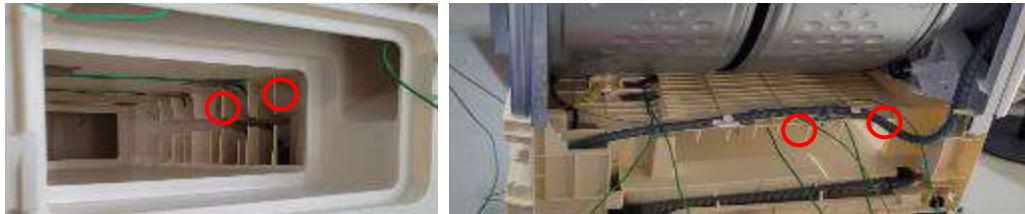
Fig. 3: Thermocouple Positions of Cooling Air Condenser Inlet and Outlet
