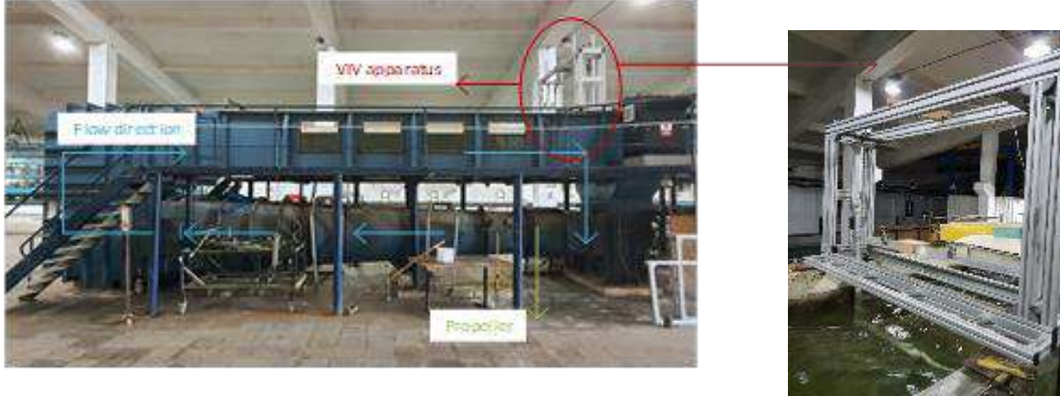
Fig. 1: ITU Naval Architecture and Ocean Engineering Building Ata Nutku Ship Model Testing Laboratory the circulation channel
