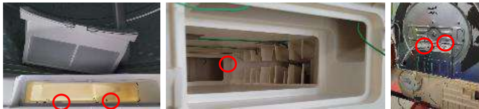
Fig. 4: Thermocouple Positions of Drying Air Condenser Inlet, Outlet and Heater Outlet
