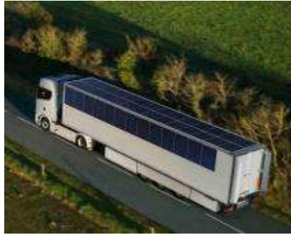
Fig. 1: Solar energy assisted cooling system on refrigerated trailer
