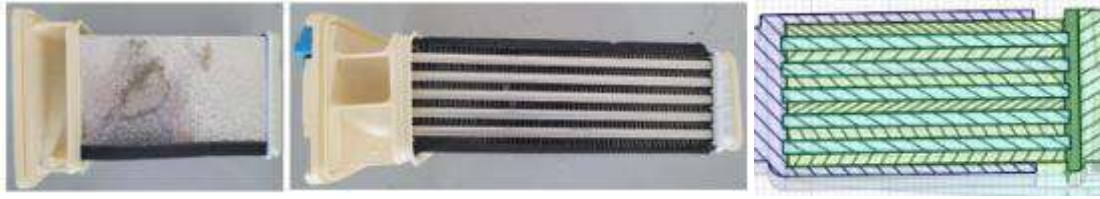
Fig. 7: Condenser and Condenser Model for CFD
