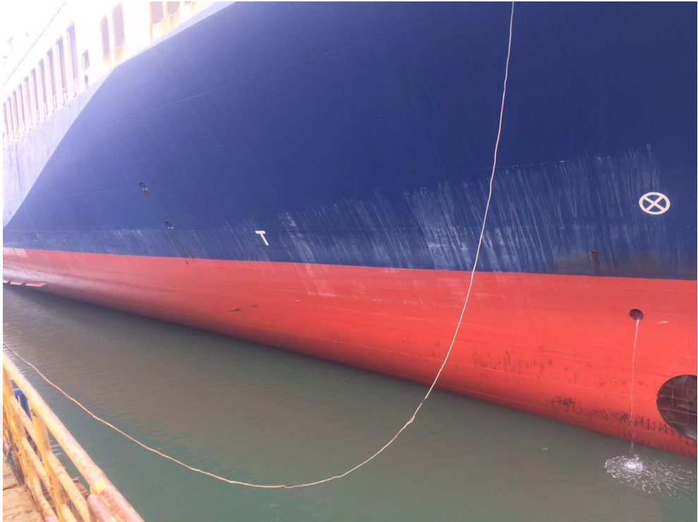
Figure 4.16. VESSEL 2, 2017 Dry-dock, photo of hull condition, condition just after entering the dry-dock
