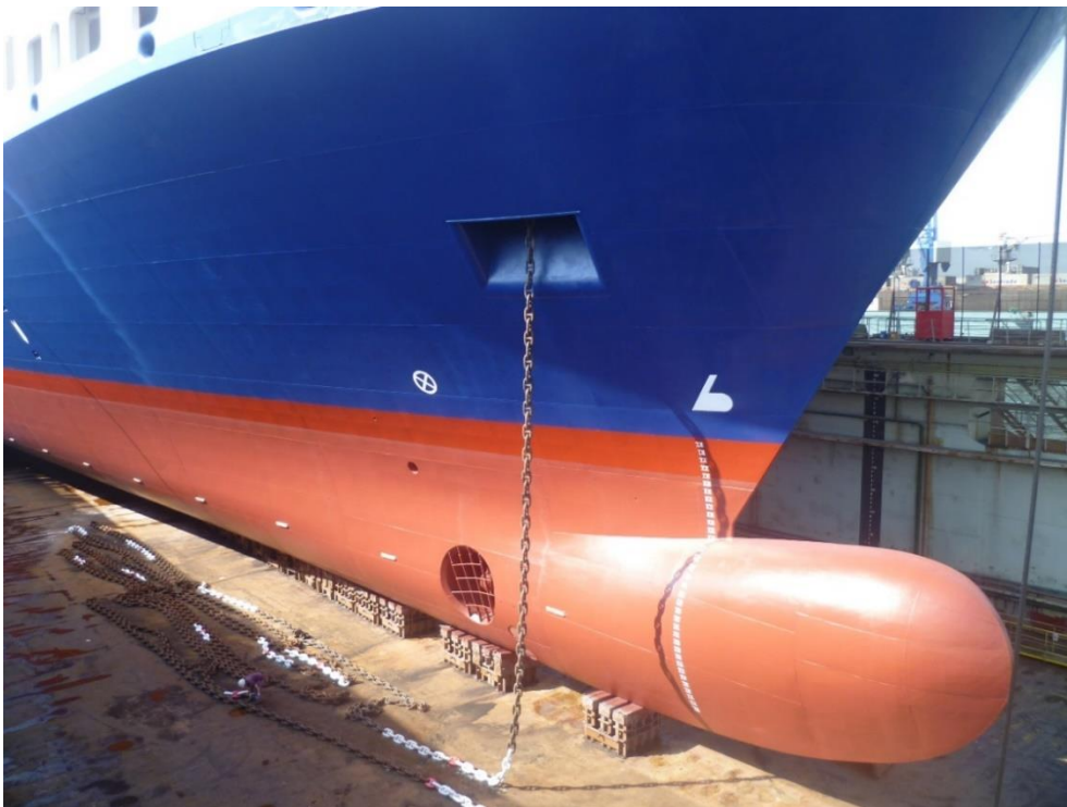
Figure 4.66. VESSEL 8, 2013 Dry-dock, photo of hull condition, after 5 th type self-polishing coating technology application
