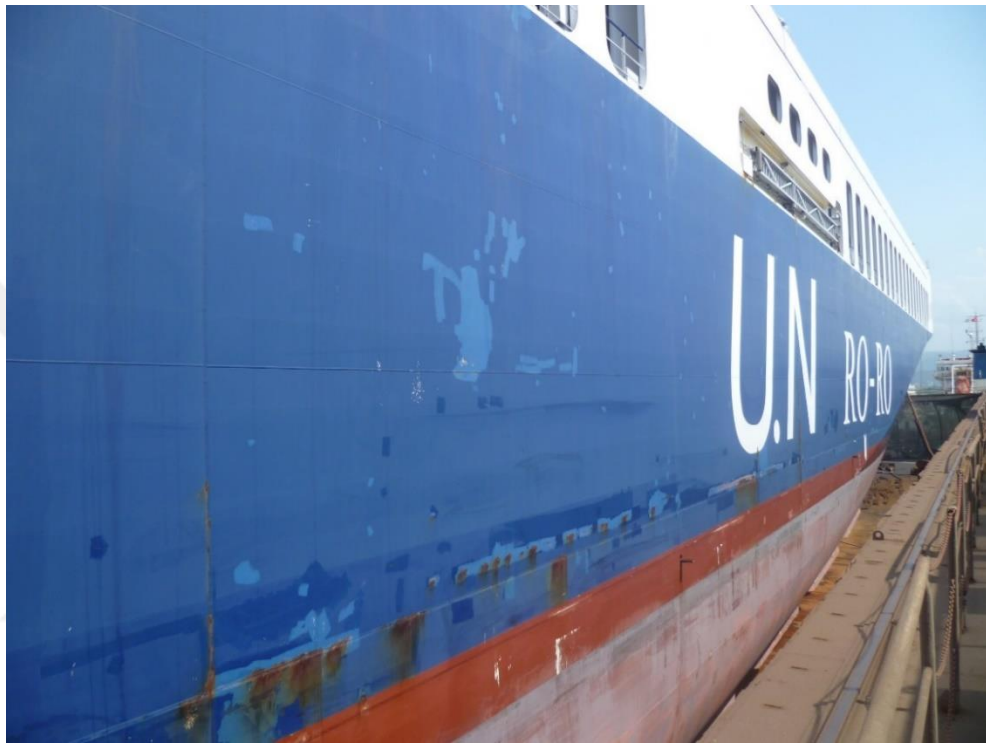
Figure 4.64. VESSEL 8, 2013 Dry-dock, photo of hull condition, after high pressure wash
