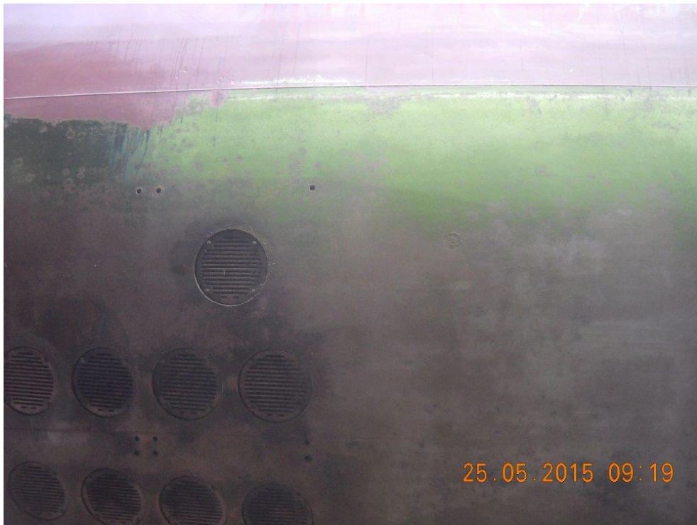
Figure 4.44. VESSEL 5, 2015 Dry-dock, photo of hull condition, before high pressure water wash
