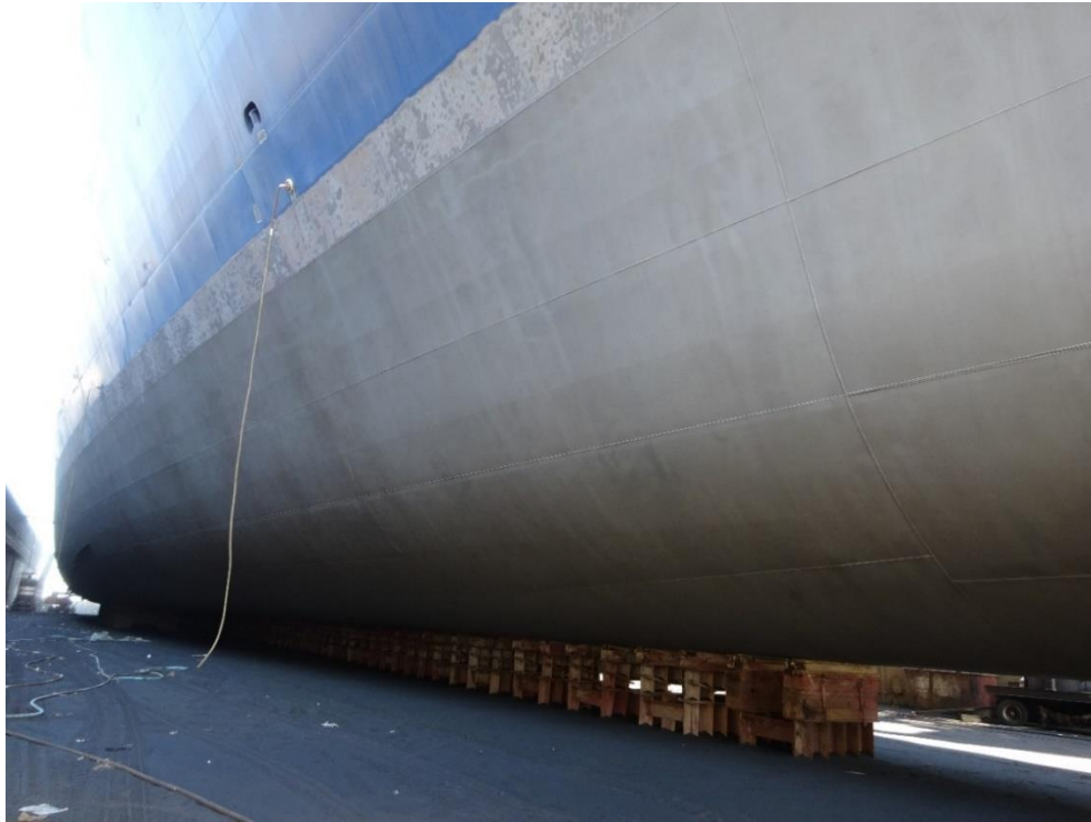
Figure 4.35. VESSEL 4, 2015 Dry-dock, photo of hull condition, full blasting completed
