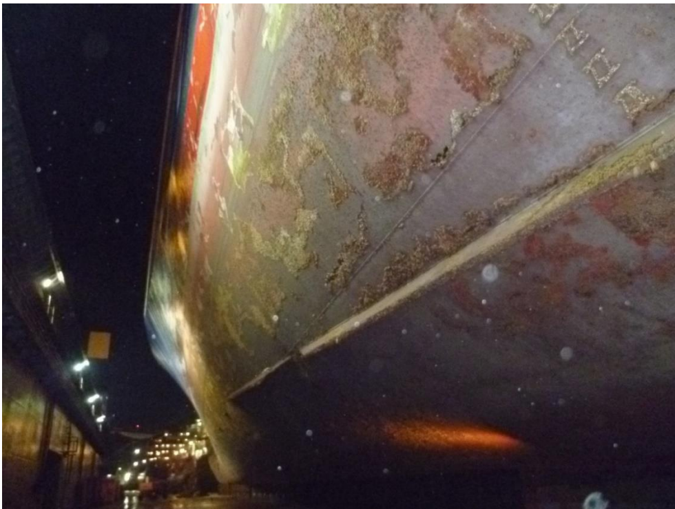
Figure 4.2. VESSEL 1, 2013 Dry-dock, photo of hull condition, after first wash, condition before 1 st type foul release coating application
