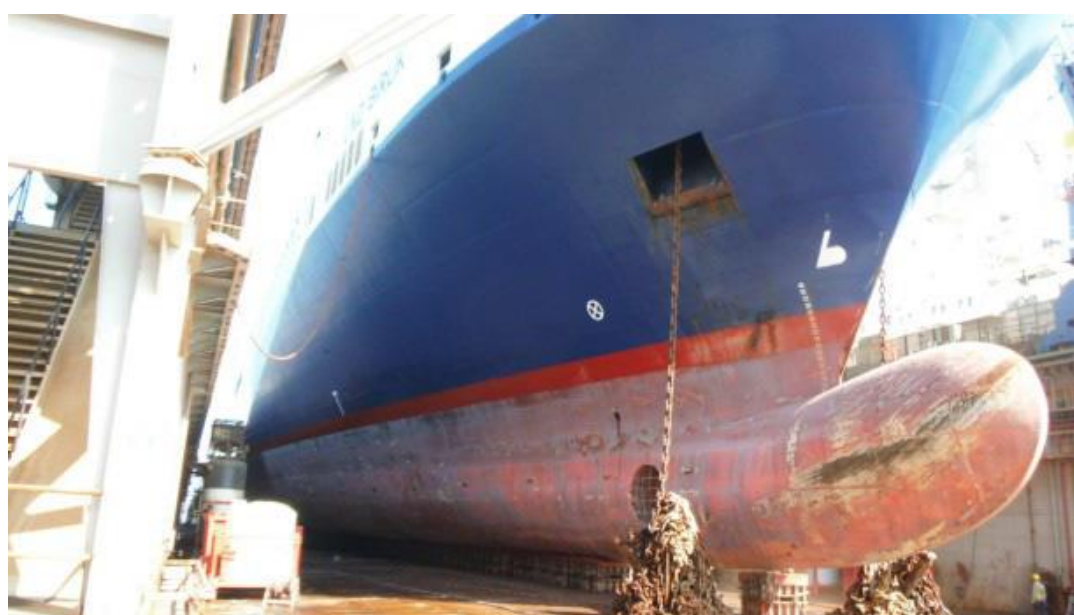
Figure 4.9. VESSEL 2, 2014 Dry-dock, photo of hull condition, after first wash, condition before 1 st type foul release coating application
