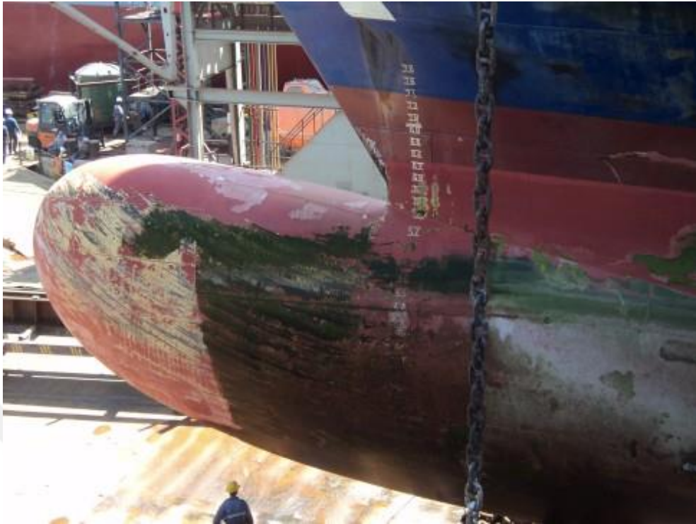
Figure 4.33. VESSEL 4, 2015 Dry-dock, photo of hull condition, during high pressure wash
