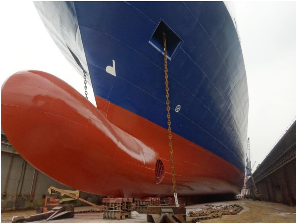
Figure 4.55. VESSEL 6, 2015 Dry-dock, photo of hull condition, after 1 st type foul release coating application
