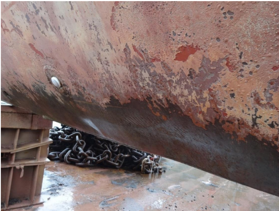
Figure 4.51. VESSEL 6, 2015 Dry-dock, photo of hull condition, after high pressure water wash
