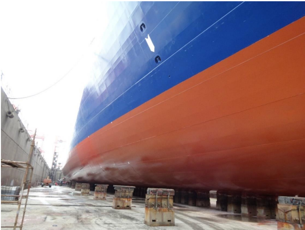
Figure 4.74. VESSEL 8, 2016 Dry-dock, photo of hull condition, full blasting + after 1 st type foul release coating application
