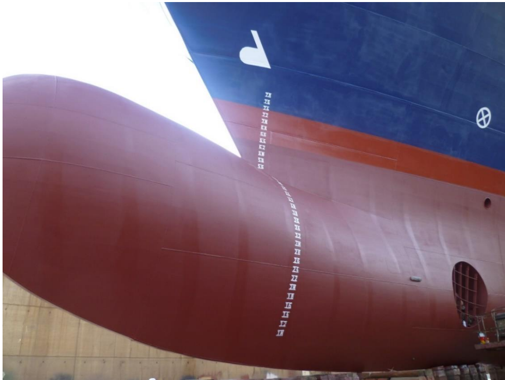
Figure 4.41. VESSEL 5, 2013 Dry-dock, photo of hull condition, after application of 3 rd type self-polishing coating
