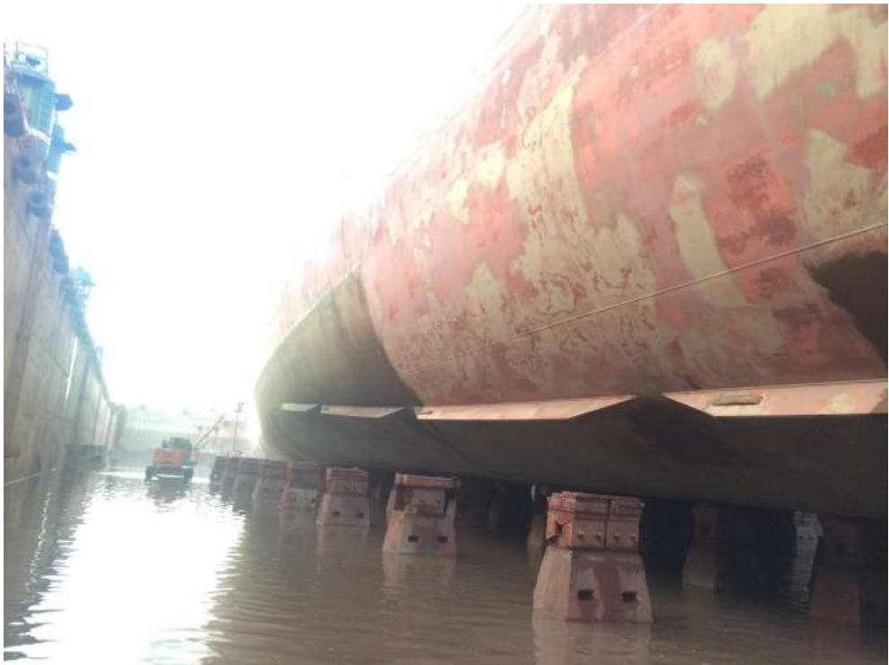
Figure 4.61. VESSEL 7, 2016 Dry-dock, photo of hull condition, during high pressure wash
