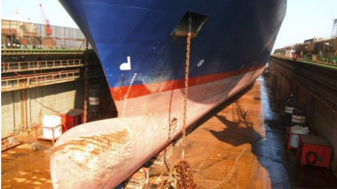
Figure 4.10. VESSEL 2, 2014 Dry-dock, photo of hull condition, after first wash, condition before 1 st type foul release coating application
