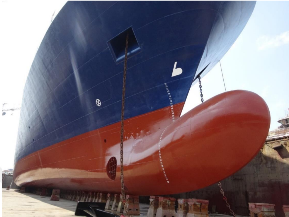
Figure 4.7. VESSEL 1, 2016 Dry-dock, photo of hull condition, condition after 1 layer of 1 st type foul release coating application
