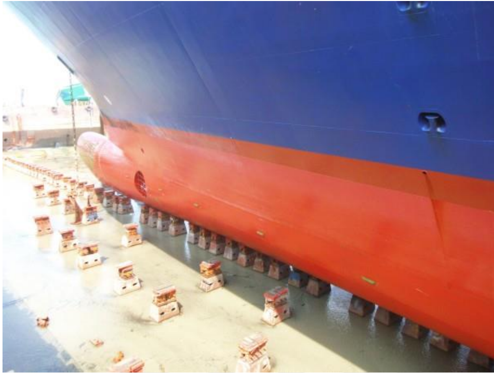
Figure 4.5. VESSEL 1, 2016 Dry-dock, photo of hull condition, just after entering the dry-dock
