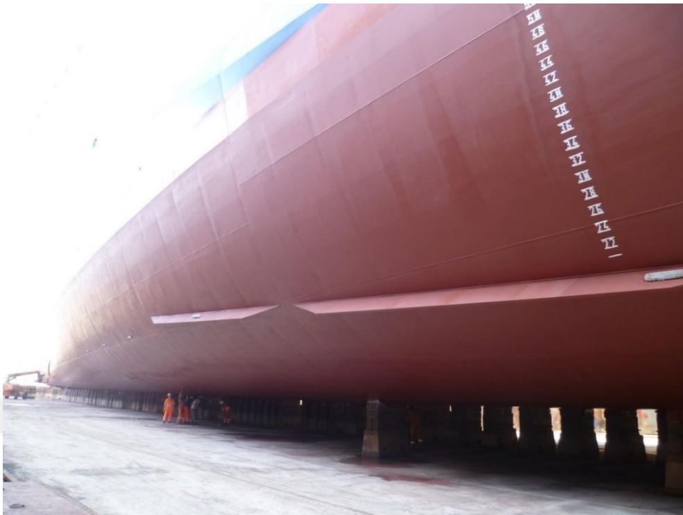
Figure 4.42. VESSEL 5, 2013 Dry-dock, photo of hull condition, after application of 3 rd self-polishing coating
