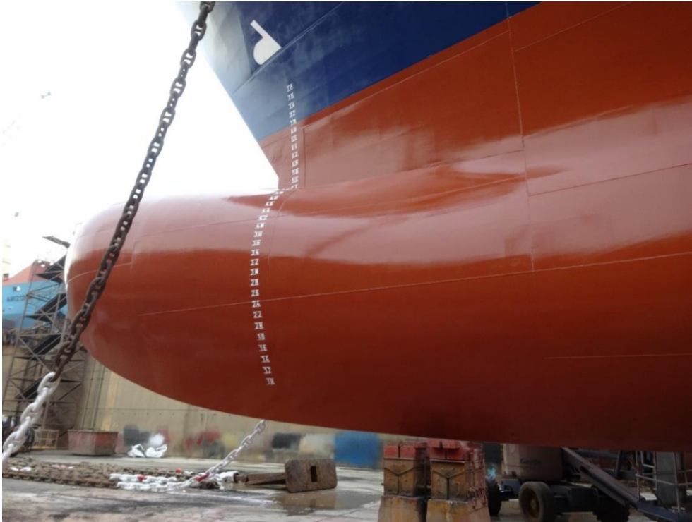
Figure 4.73. VESSEL 8, 2016 Dry-dock, photo of hull condition, full blasting + after 1 st type foul release coating application
