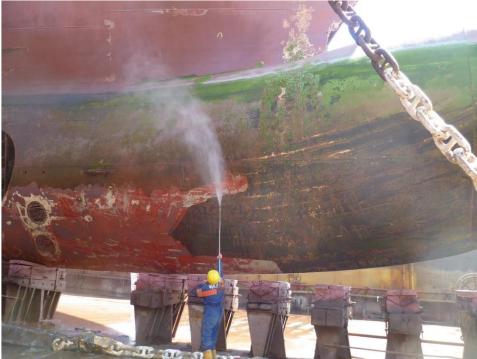
Figure 4.28. VESSEL 4, 2013 Dry-dock, photo of hull condition, condition during first wash with fresh water
