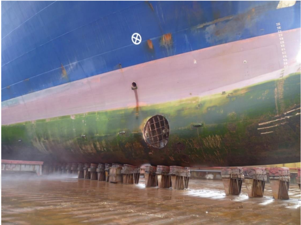
Figure 4.48. VESSEL 6, 2013 Dry-dock, photo of hull condition, just after entering the dry-dock
