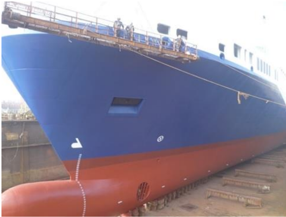
Figure 4.31. VESSEL 4, 2013 Dry-dock, photo of hull condition, condition after full blasting + 2 nd type self-polishing coating application
