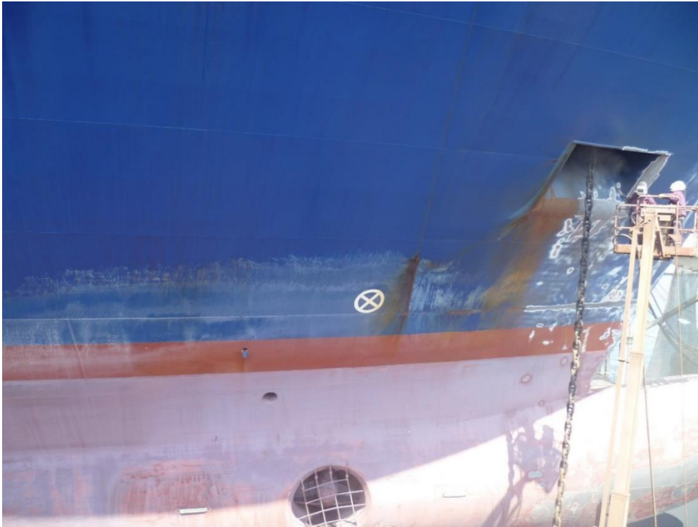
Figure 4.65. VESSEL 8, 2013 Dry-dock, photo of hull condition, after high pressure wash
