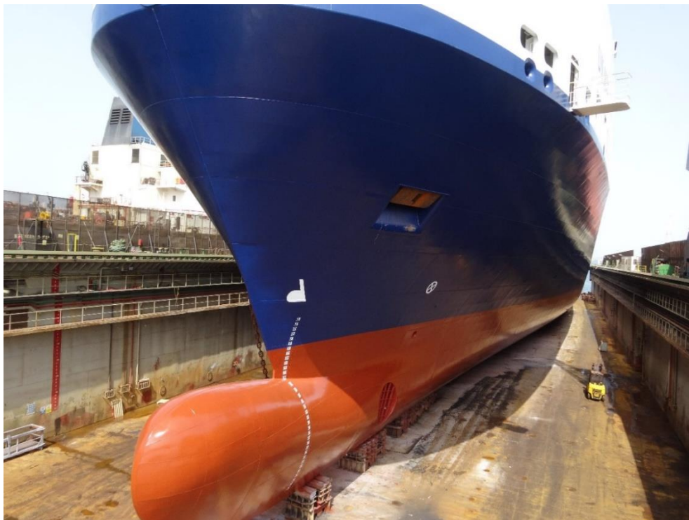
Figure 4.36. VESSEL 4, 2015 Dry-dock, photo of hull condition, after 1 st type foul release coating application
