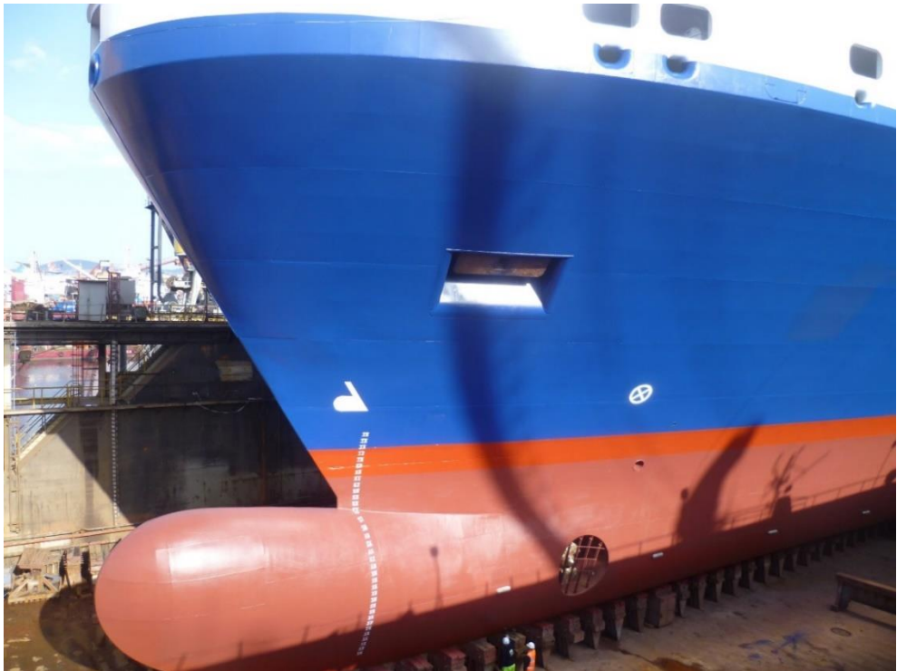
Figure 4.20. VESSEL 3, 2013 Dry-dock, photo of hull condition, condition after 1 st type self- polishing coating application with only %25 blasting
