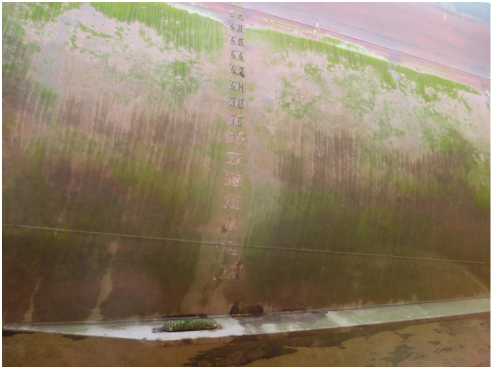
Figure 4.39. VESSEL 5, 2013 Dry-dock, photo of hull condition, just after entering the dry-dock
