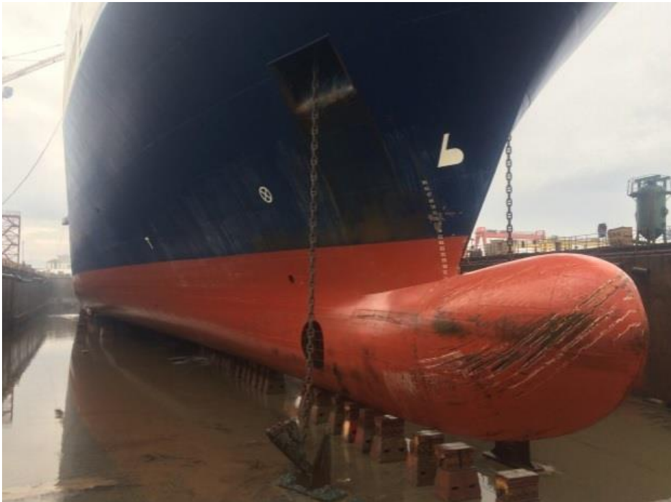
Figure 4.15. VESSEL 2, 2017 Dry-dock, photo of hull condition, condition just after entering the dry-dock
