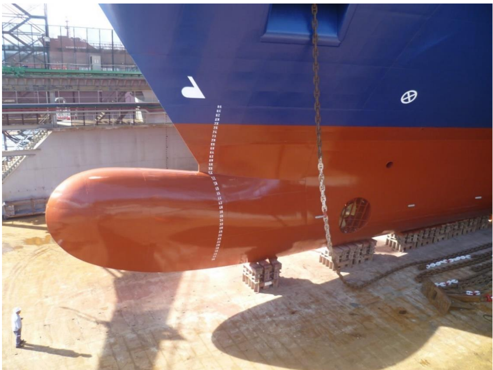
Figure 4.4. VESSEL 1, 2013 Dry-dock, photo of hull condition, condition after 1 st type foul release coating application
