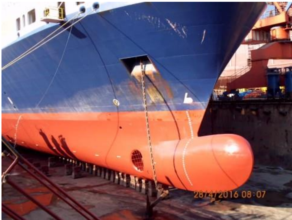
Figure 4.63. VESSEL 7, 2016 Dry-dock, photo of hull condition, after 4 th type self-polishing coating application
