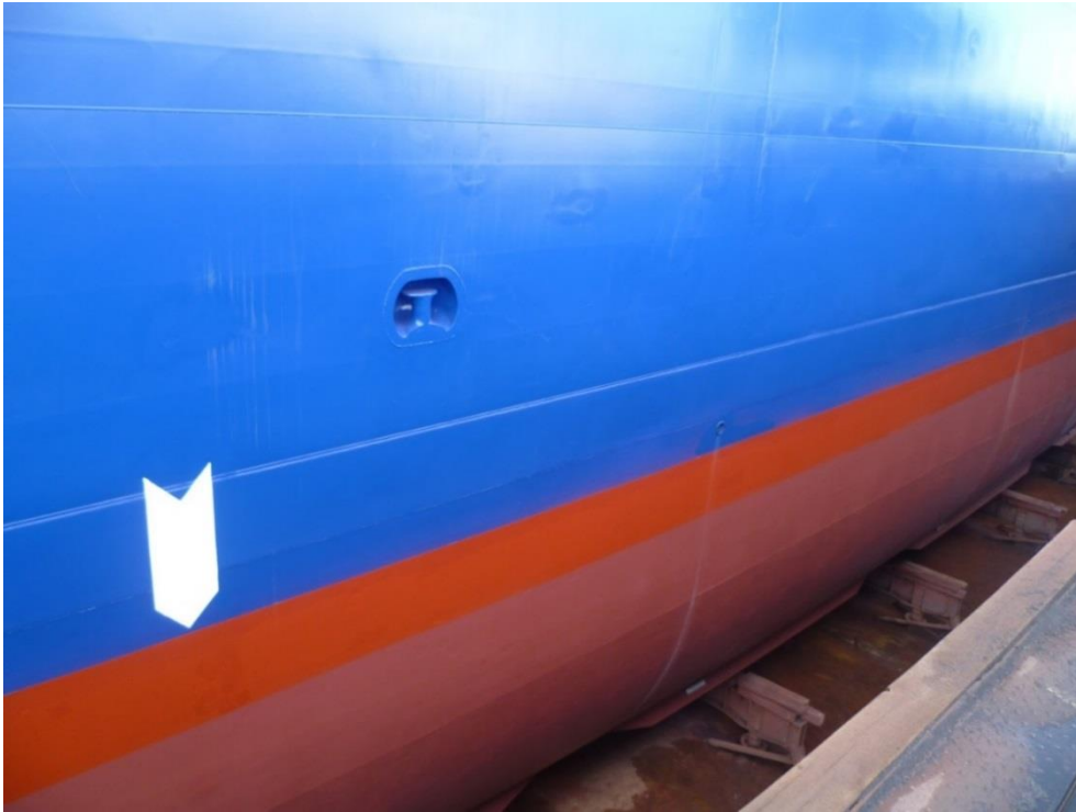
Figure 4.50. VESSEL 6, 2013 Dry-dock, photo of hull condition, after 1 st type self-polishing coating application
