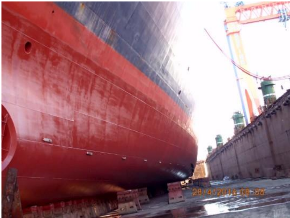
Figure 4.62. VESSEL 7, 2016 Dry-dock, photo of hull condition, after 4 th type self-polishing coating application
