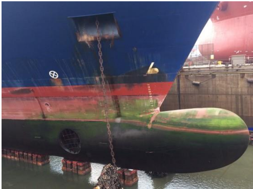
Figure 4.72. VESSEL 8, 2016 Dry-dock, photo of hull condition, just after entering the dry-dock
