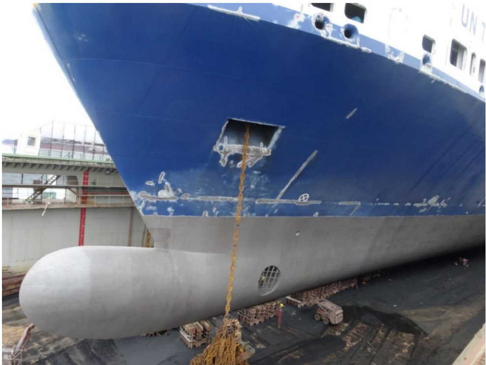
Figure 4.53. VESSEL 6, 2015 Dry-dock, photo of hull condition, after full blasting
