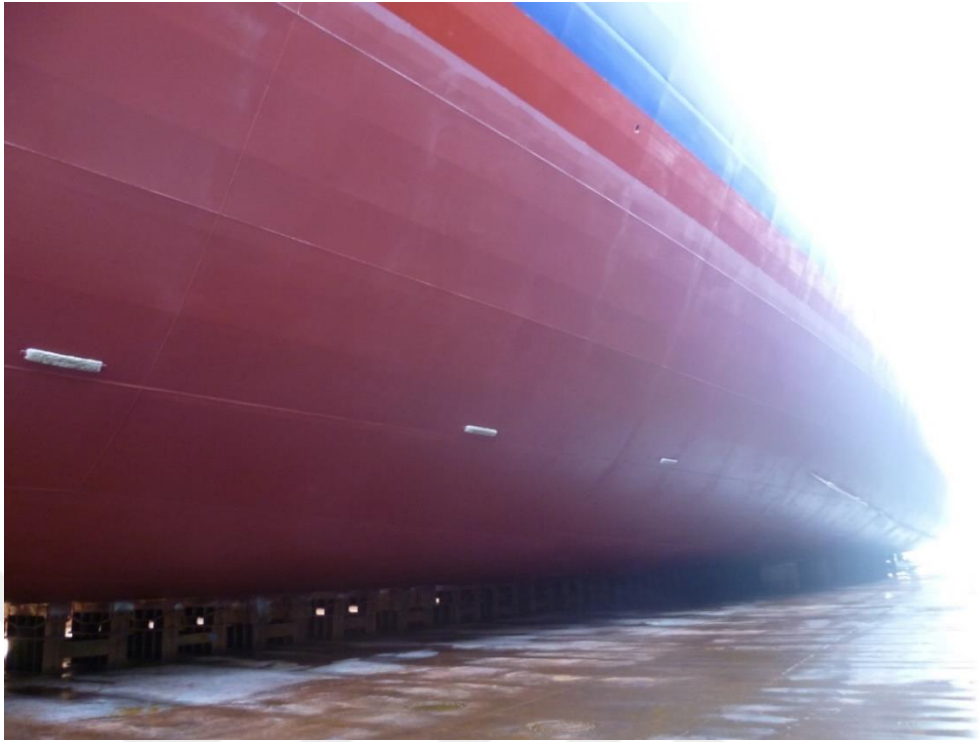
Figure 4.67. VESSEL 8, 2013 Dry-dock, photo of hull condition, after 5 th type self-polishing coating technology application
