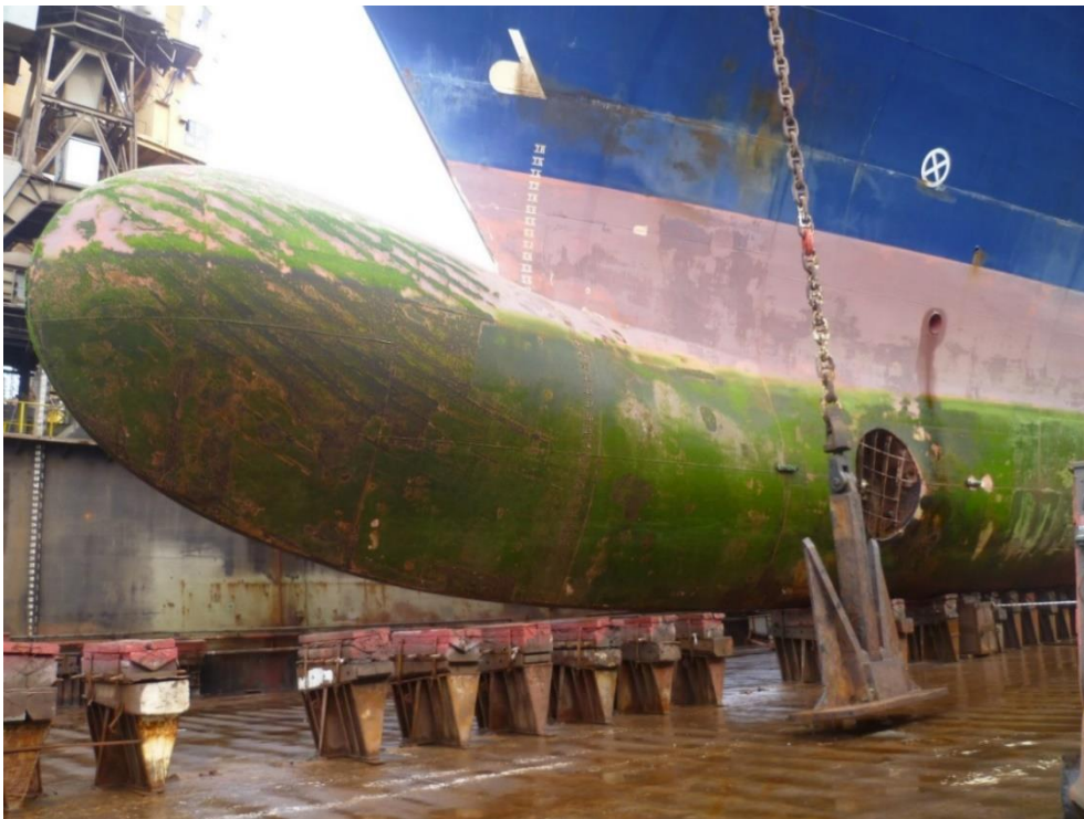
Figure 4.47. VESSEL 6, 2013 Dry-dock, photo of hull condition, just after entering the dry-dock
