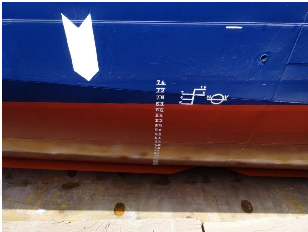
Figure 4.37. VESSEL 4, 2015 Dry-dock, photo of hull condition, after 1 st type foul release coating application
