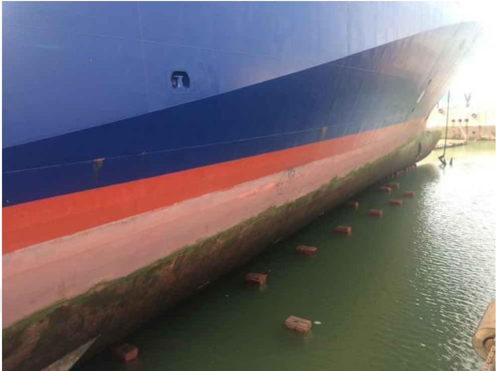
Figure 4.60. VESSEL 7, 2016 Dry-dock, photo of hull condition, just after entering the dry-dock
