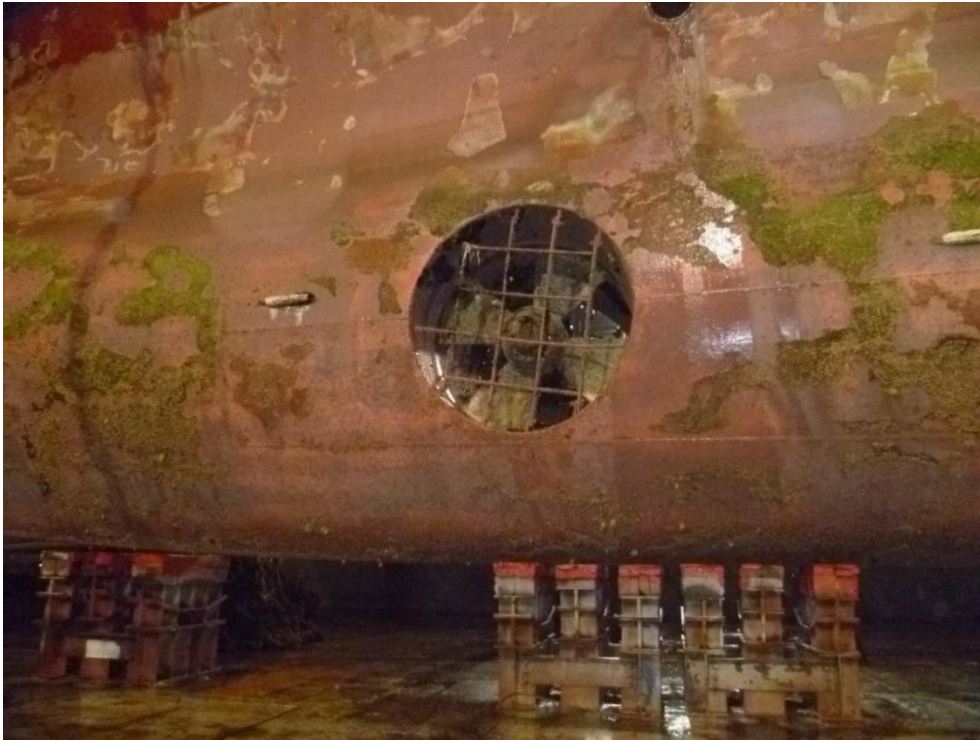
Figure 4.1. VESSEL 1, 2013 Dry-dock, photo of hull condition, after first wash, condition before 1 st type foul release coating application
