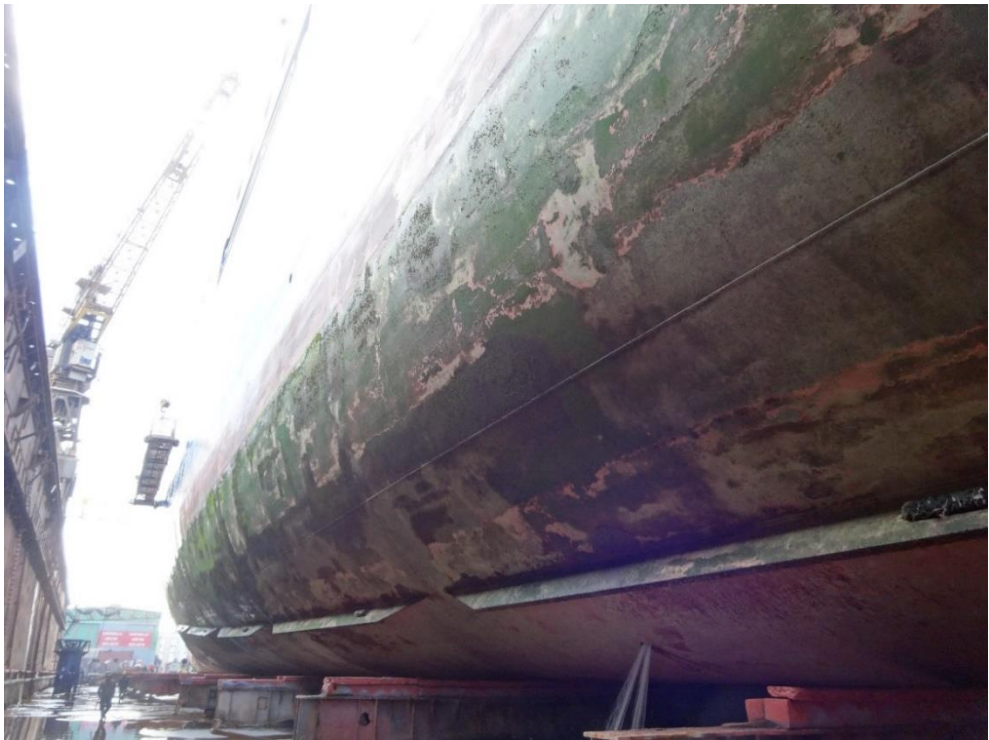
Figure 4.24. VESSEL 3, 2015 Dry-dock, photo of hull condition, just after entering the Dry-dock
