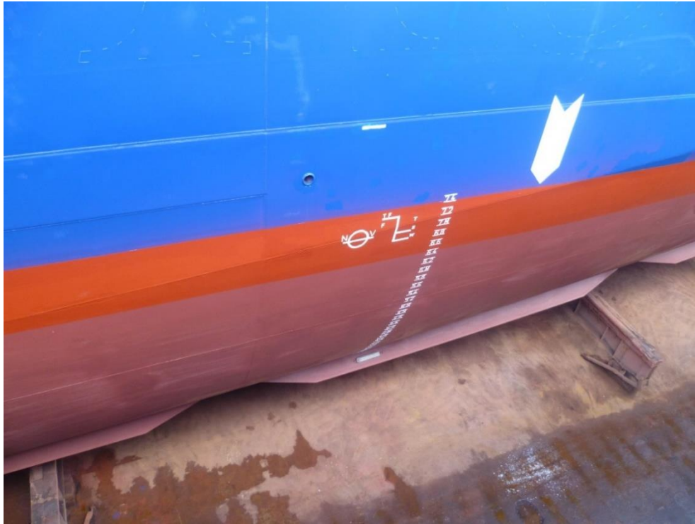
Figure 4.21. VESSEL 3, 2013 Dry-dock, photo of hull condition, condition after 1 st type self-polishing coating application with only %25 blasting
