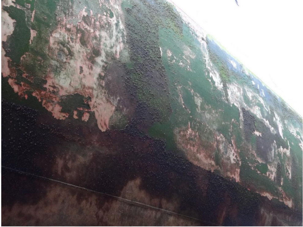
Figure 4.23. VESSEL 3, 2015 Dry-dock, photo of hull condition, just after entering the Dry-dock
