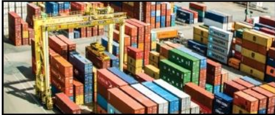
Figure 5.15. An RTG in use for stacking containers. (Source: http://tfdbrazil.com.br/?page_id=110 )
