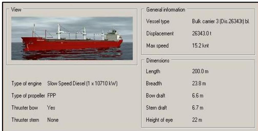
**Figure 5.7.** Ship model used in simulation
