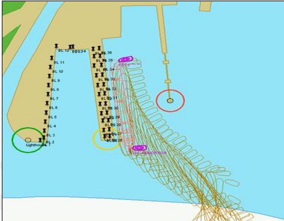
**Figure 5.10.** Tracks created by the ship during coming alongside
