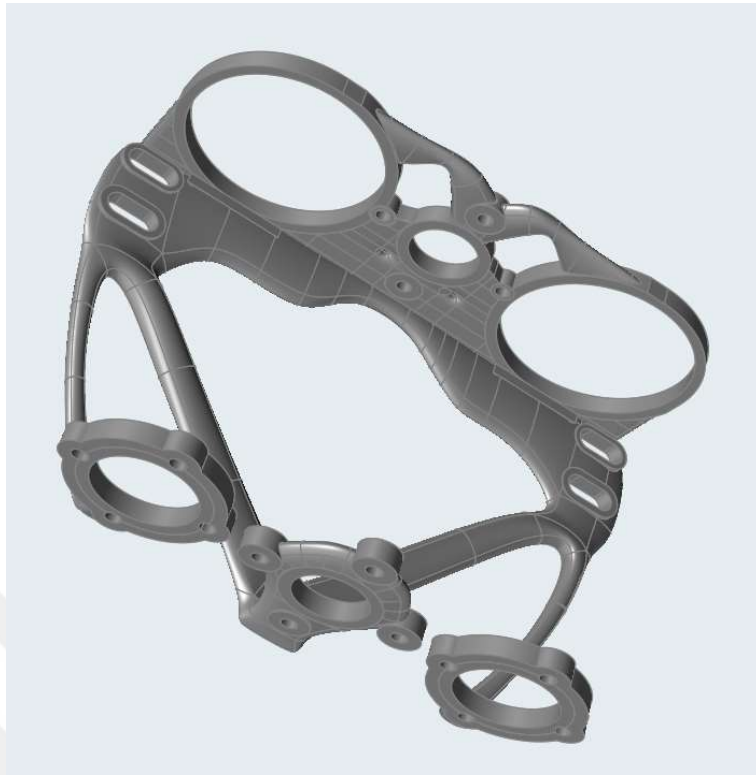
Figure 5-11 Another view of Redesigned Model with the use of PolyNURBS
