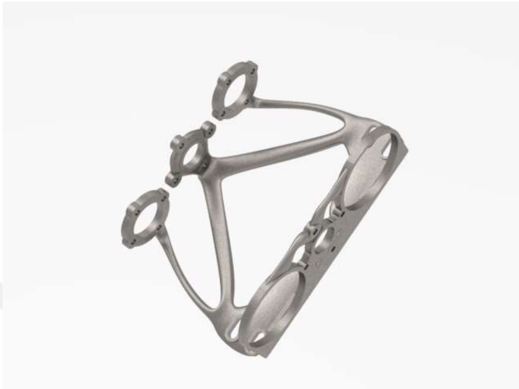
Figure 5-12 Realistic Image of Redesigned Model After Rendering in Evolve Software
