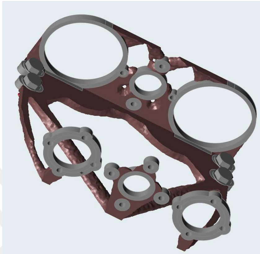
Figure 5-7 Part After Topology Optimization Run
