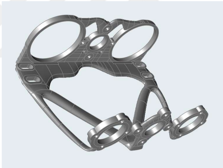
Figure 5-10 Redesigned Model with the Use of PolyNURBS
